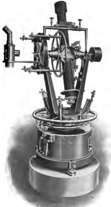
FIG. 25. — A 5-inch Altazimuth By Warner & Swasey
